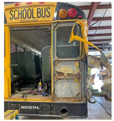
Before and after pictures of one of our older buses found to require rust repair. The work was completed in-house by our mechanics, Ben and Caleb.
